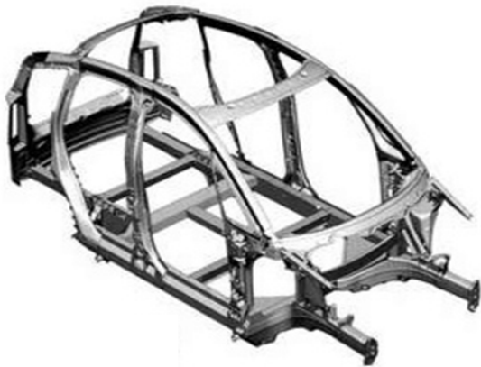
ALUMINIUM BODY IN WHITE OF AUDI A2
