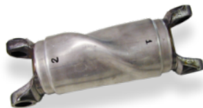
HIGH PERFORMANCE: In testing, the mother material will surrender prior to the weld area
